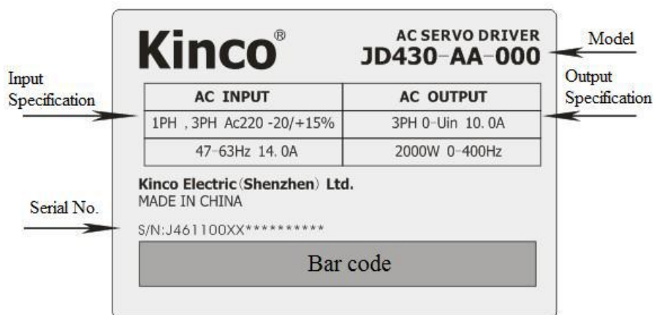
Fig. 1-1 Nameplate of a servo driver
