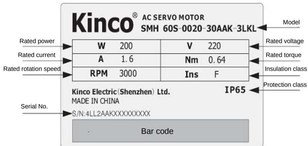
Fig. 1-2 Nameplate of a servo motor
