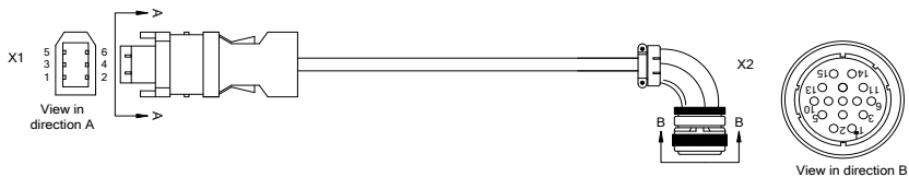
Figure 4-10 Absolute encoder motor wiring
